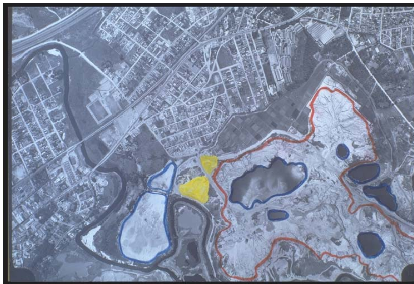
Photo 1- Sand mining (pit: red; stocking: yellow; tailing dams : blue) in Itaquaquetuba city, RMSP.
